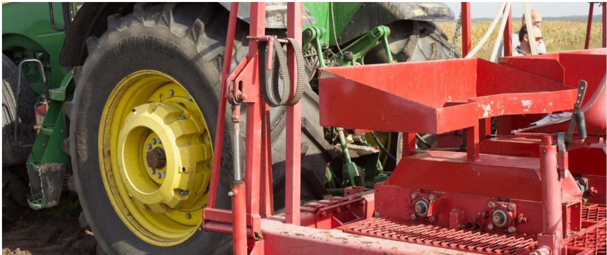
FIGURE 4 A tractor for the mechanical planting of a willow SRC field in the Ukrainian case study site
