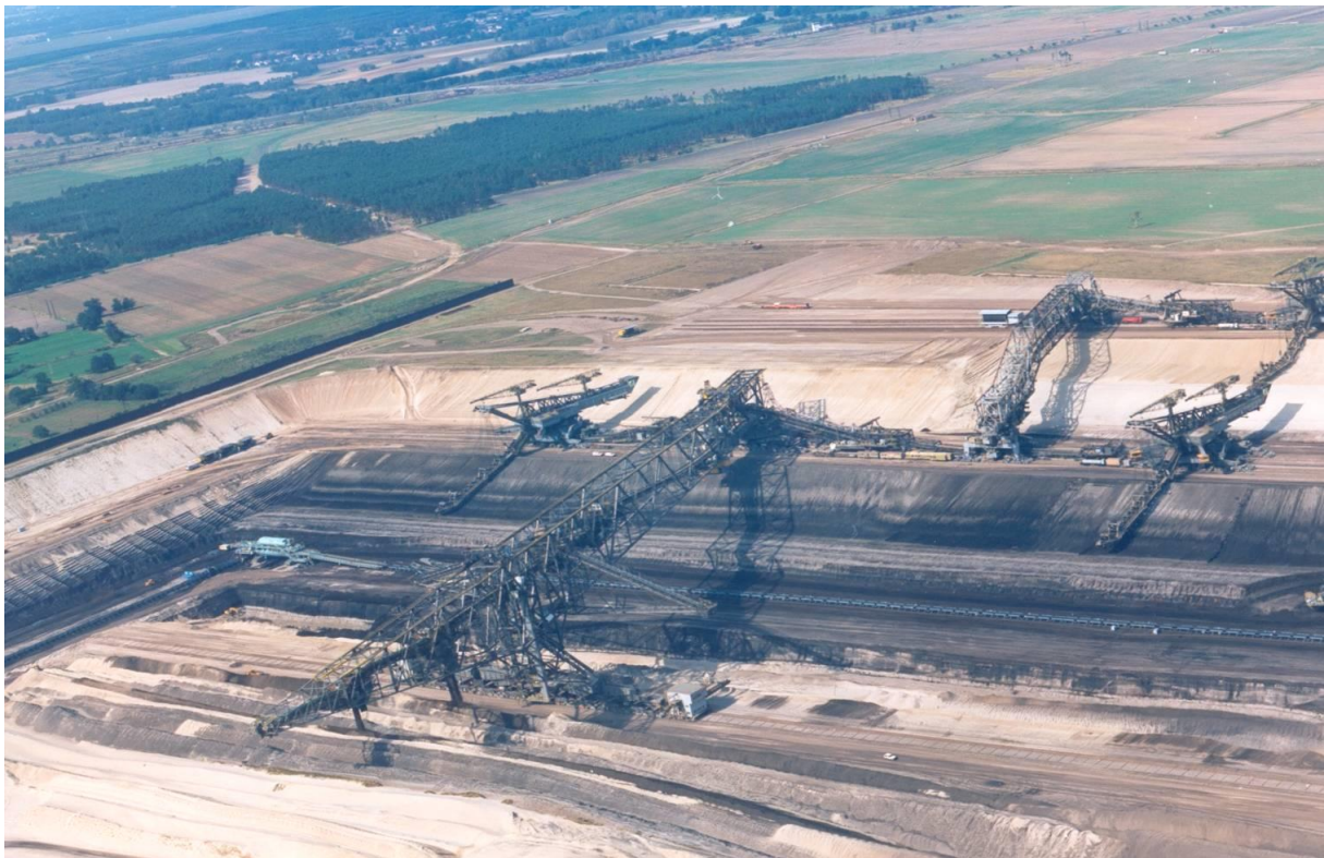
FIGURE 9: OVERBURDEN CONVEYOR BRIDGE F 60 AT THE OPENCAST MINE JÄNSCHWALDE - THE LARGEST MOVABLE MACHINE IN THE WORLD
